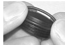
Fig. 152 - TMT O-RING INSTALLATION
