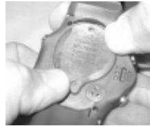
Fig. 151 - ALT BATTERY HATCH INSTALLATION
