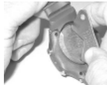
Fig. 150 - ATOM BATTERY HATCH INSTALLATION
